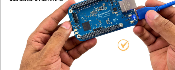
Fig. 2.7: Connecting BeagleV-Ahead to flash eMMC
