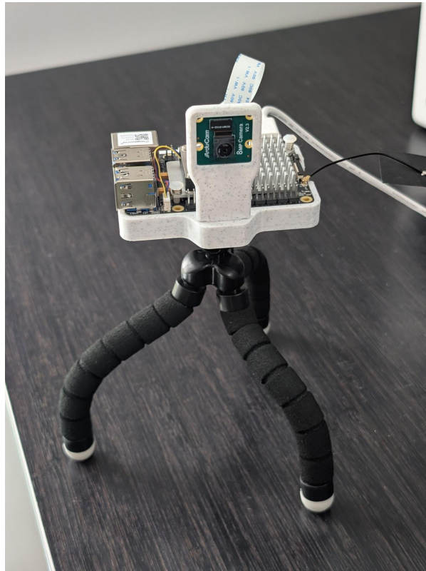
Fig. 5.29: IMX219 CSI camera module + 3D printed camera mount
