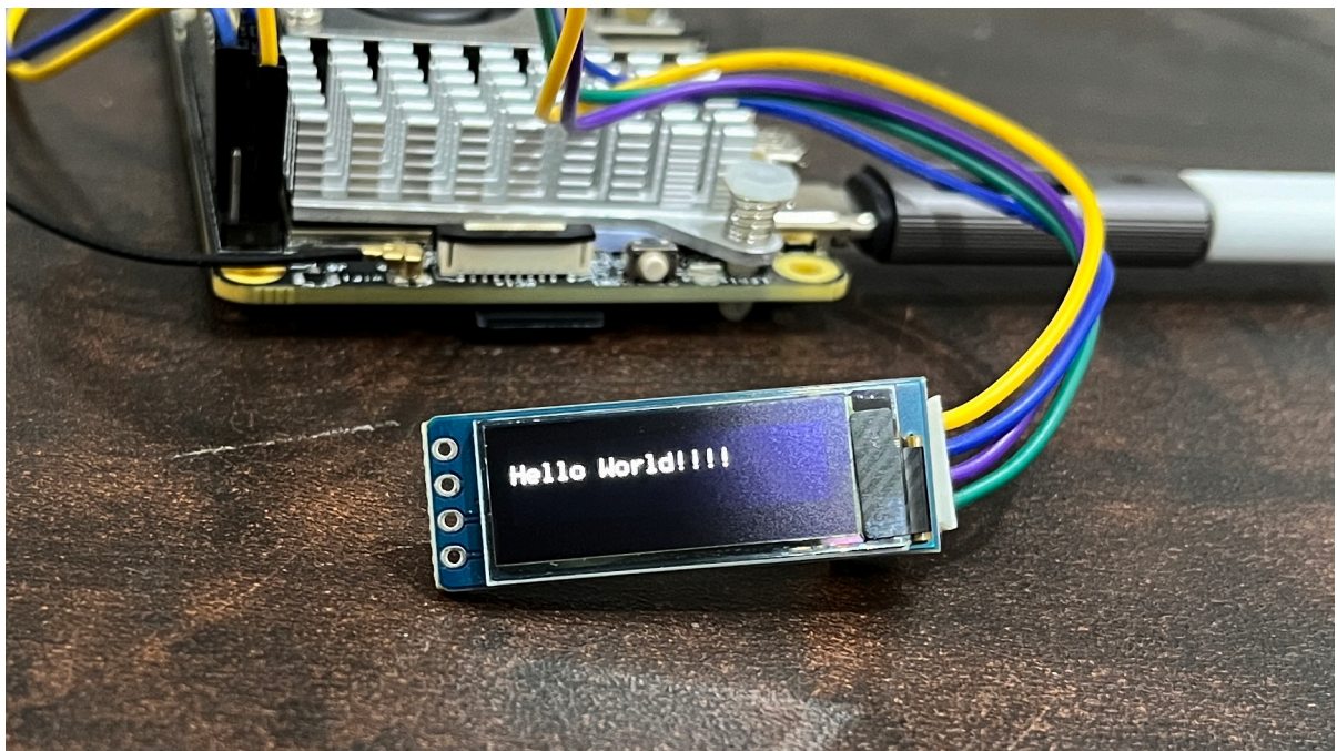
Fig. 5.22: Hello World!!!! on 128x32 OLED
